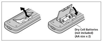
Open the battery compartment on the back of the remote control, and insert the batteries, taking care to align the  $\bigoplus$  and  $\bigoplus$  polarities.
