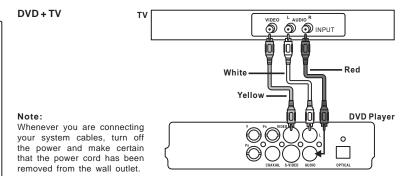
1. Connect the audio cables to the AUDIO OUT L and R jacks on the back of your DVD player and to the corresponding AUDIO INPUT jacks on your TV.
