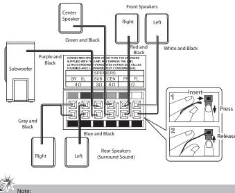
When connecting the speakers, make sure the polarities ("+" speaker wire to "+" on the receiver) of speaker wires and terminals match. For example, red wire to red terminal on the receiver. If the cords are reversed, the sound will be distorted. Do not let the speaker wires touch each other, it will damage the system's amplifier
