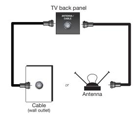
Connect your regular cable to the TV's ANTENNA/CABLE INPUT to receive analog channels or connect an antenna to the TV's ANTENNA/CABLE INPUT to receive off-air local digital and analog channels.
