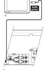
Connect a stereo audio cable (not supplied) from the audio outputs of your TV to the **TV IN** jacks on this system.
