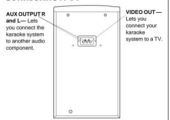
To see the words from a karaoke video cassette or CD/CDG on a TV or monitor, plug one end of the supplied cable into the karaoke system's **VIDEO OUT** jack and the other end into your TV or monitor's VIDEO IN jack.
