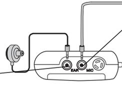
**MIC Jack** — lets you connect an optional dynamic microphone with a 1/8-inch (3.5mm) plug to extend the recording range. The built-in microphone automatically disconnects.
