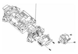
11 If you have installed the All Wheel Drive kit: Remove the center gear and the center shaft and replace the small bearing. Tweezers may be helpful for this step.
