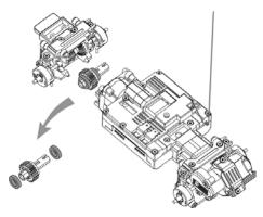
Restore the front differential gear unit as shown in the illustration.
