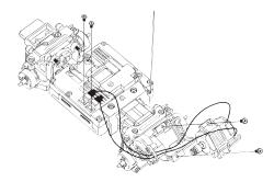
Remove the two screws on the rear drive unit to remove the rear gear case. Then, remove the differential gear and the third gear.
