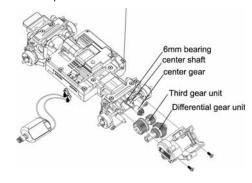
12 Place the center gear back on the center shaft. Lightly press and rotate the center gear so the flat side of the center shaft and the center gear mesh.
