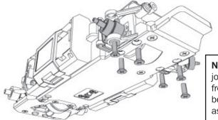
**Note:** Be sure the universal joints have not disengaged from the differential axles before screwing the assembly into place.
