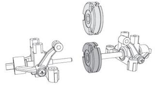
Reassemble the rear section of your car in reverse order. Reassemble the front and rear **dampers** and **wheels**.
