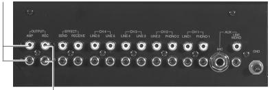
**OUTPUT AMP L/R** — use an audio patch cord (not supplied) to connect your receiver or amplifier to your mixer (match left to left, right to right). The sound is output to your stereo sound system.
