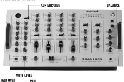
We recommend adjusting **GAIN** before presetting the inputs since some sound imbalance could occur.
