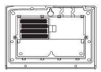
Close the cover and secure it with the screw. If you are replacing the batteries, reconnect the phone line and the phone.
