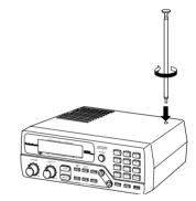
The antenna's length controls its sensitivity. Adjust the length of the telescoping antenna as follows for the best reception.
