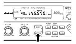
If the scanner is scanning and stops at the desired channel, press MANU-AL once. Repeatedly press MANUAL to step through the channels one at a time.
