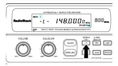
To clear a single frequency from skip memory so the scanner can stop on it during a limit, direct, or weather search, press **LIMIT** to hold the search, press D or — to select the skipped frequency, then press **L/O/ SEARCH SKIP** until **LOCKOUT** disappears.
