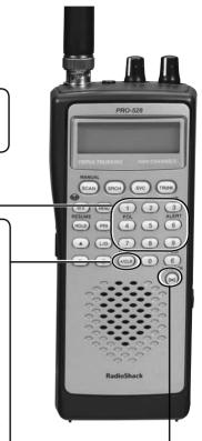
→ • F /KEYLOCK — locks the keypad to prevent changes; turns the display and key backlight on and off.
