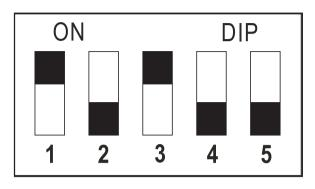
Dip switches 1 to 4 are for channel selection. Switch 5 lets you set up the auto-sequence timer for four cameras on four different channels to monitor a series of rooms for maximum supervision of the house (or office).  $\mathcal{Y}$
