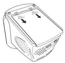
3. Install 10 C cell batteries (not supplied) according to the battery polarities marked inside the compartment.
