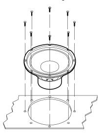
Install the speaker from the cabinet front (with the terminals at the bottom of the speaker) and keep it flush with the baffle face. Secure the speaker with eight screws (not supplied).
