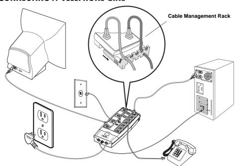
Connect one end of a modular telephone cord (not supplied) to the surge protector's FAX/MODEM IN jack, and the other end to a telephone wall jack.
