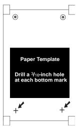
> 3. Press a plastic anchor into the hole at each bottom mark and tap the anchor into the wall with a hammer until the anchor is seated.
