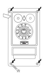
For additional stability, you can also use the supplied rubber spacers in addition to the screws. After you insert the screws through the phone's mounting holes, place a rubber spacer over each screw, so the spacer is between the back of the phone and the wall, then place the phone against the wall
