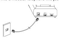
If you use two single-line jacks, you must connect the lines with an optional two-line coupler (such as RadioShack Cat. No. 279-401).
