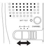
**Note**: Your TRC-235 comes with Channel 14 crystals installed in channel position A. To use other channels, you must first install crystals in channel positions B and C inside the TRC-235 (see "Adding Crystals" on Page 24).
