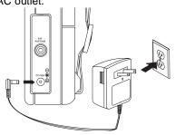
It takes about 20 hours to charge new or fully discharged nickelcadmium batteries. Subsequent charges take about 14 to 16 hours.
