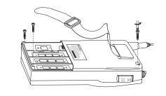
**Caution:** The **BATT TEST** button might come off of the front of the TRC-235 when you remove the front cover. If this happens, simply replace it.
