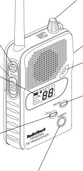
To turn the radio on or off, hold down **POWER** for about 1 second.
