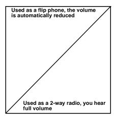
**Important:** Do not hold the radio's speaker against your ear with this key cover closed. The radio is automatically set to a high volume when the key cover is closed.
