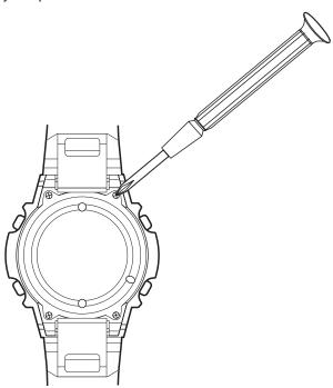
2. Use a flat-blade screwdriver to gently pry off the metal clip.
