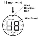
The wind speed and wind direction are updated continuously until the gauge is manually stopped or until it times out (90 seconds). The wind direction icon disappears if no valid direction is received in three seconds.
