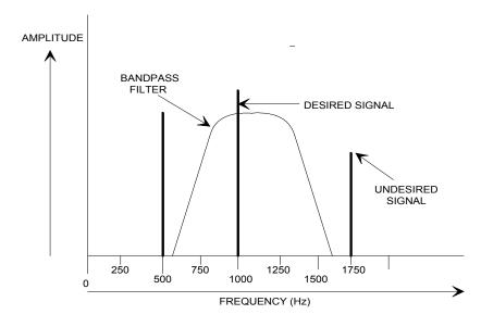
The audio filter board creates an audio frequency bandpass filter to remove the undesired tones. It also has a selectable bandwidth (the width of the bandpass filter) of 100, 250, 500, or 750 Hz. The center frequency of this filter is also tunable from 400 - 1000 Hz, so you can tune the radio to frequency that you would like to hear, not to whatever frequency the filter wants to "listen to".
