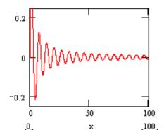
The effect is an exponentially decaying sine wave. An NE555 timer provides the "striker" that gets the oscillator going. Every second or so the NE555 outputs a pulse that appears at the junction of R10 and R5. Then Q1 outputs the waveform above which is fed to an audio amplifier. The result is an output that sounds like a faucet drip or sometimes maybe a guitar string pluck.
