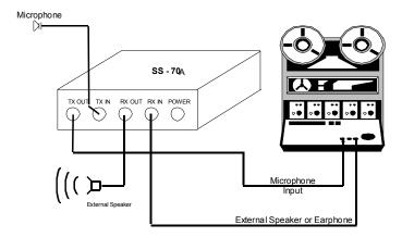
Once the wires are "hooked up", energize the circuit and try taping a scrambled message. Then try to playback and descramble it! While playing
