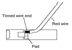
up. The motors are a little sensitive to the heat and can't be baked to death like most other components. Solder the black wire to the other pad, and then repeat this whole process for the other motor.
