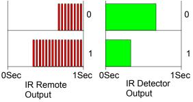
the one second time frame (0.60 sec.) of it. For a 0, the LED will be switched on and off at 38 kHz for 30% of the time (0.30 sec.) of the entire second.
