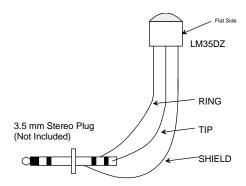
Remember that the temperature sensing circuitry is relying on a very small voltage measurement to determine the temperature, so use a good quality shielded cable for remote sensing applications.
