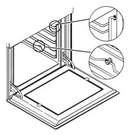
The shelf support can then be hinged upwards and lifted from the mounting holes in the upper corners of the oven prior to removal.
