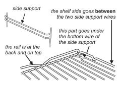
The shelf supports are numbered from 1-5 in the main oven and 1-3 in the top oven, position 1 being the lowest.
