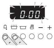
Press and hold as above. At the same time, press (-) or (+) until the correct time shows. Don't forget it's a 24 hour clock. If you make a mistake or press the wrong button, turn off the power supply for a minute or two and start again.
