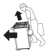
Do not use the door handles or control knobs to manoeuvre the cooker. Use the hotplate and griddle bowl areas. Remove the pack base tray.
