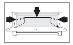
After placing your food on the grill tray pan, slide the grill pan onto the side supports just below the burners. Make sure it is pushed right in and touches the back stop.
