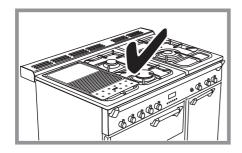
The griddle fits a single pan support, front to back. It is designed for cooking food on directly. Don't use pans of any kind on it. The griddle surface is nonstick and metal cooking utensils (e.g. spatulas) will damage the surface. Use heat resistant plastic or wooden utensils.
