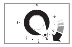
Turn the control knob back to the Mark you wish to cook on and for best results pre-heat the oven for 15 minutes before placing your dishes in it.
