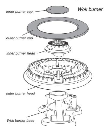
When reassembling the Wok burner, turn over the large base ring and find the 'D' shaped area.
