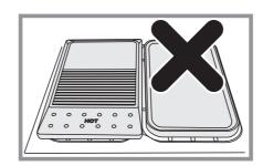
Always leave space around the griddle for the gases to escape. **Never** fit two griddles side by side. Large pans should also be spaced well apart. The maximum pan base diameter is 250mm (10in).
