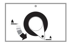
The low position, marked with the small flame symbol, is beyond high, not between high and off.
