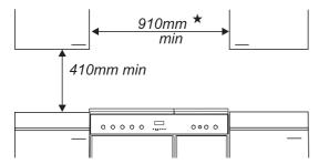
\*Any cooker hood should be installed in accordance with the hood manufacturer's instructions.
