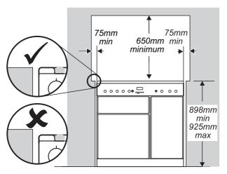
The hotplate surround should be level with, or above, any adjacent work surface. Above hotplate level a gap of 75mm should be left between each side of the cooker and any adjacent vertical surface.
