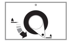
Adjust the flame height to suit by turning the knob. On this cooker the low position is beyond high, **not** between high and off. The small flame marks the 'low position'. Turn the knob towards it after the contents of a pan have boiled.
