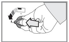
Press in the grill knob, turn to the large flame symbol (\*) and press the igniter button or light with a match.
