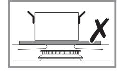
Simmering aids, such as asbestos or mesh mats, are NOT recommended. They will reduce burner performance and could damage the pan supports.
