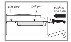
For best results preheat for 2 minutes with the grill pan in position. After placing your food on the grill pan grid, slide the grill pan onto the side supports just below the burners. Adjust the flame height to suit by turning the knob.
