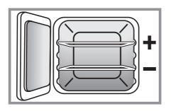
Dishes placed above the central position will be cooked at approx. one gas Mark higher, dishes cooked below approx. one gas Mark lower. You can therefore cook dishes requiring different gas Marks at the same time.
