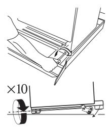
Make sure you lower BOTH REAR ROLLERS. There are two adjusting nuts, one for each roller, at both the front bottom corners of the cooker. Open the grill door and the Tall oven door. Grip under the facia panel and lift the front of the cooker.
