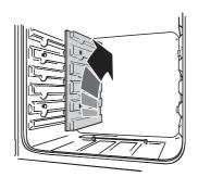
Each side of the oven is fixed with four fixing screws. You don't have to remove the screws to remove the oven linings. Lift each side panel upwards and they will slide off the screws. Then pull them forwards.
