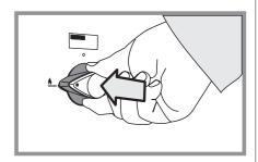
The grill has a special safety device with stops the flow of gas to the grill if the flame goes out. Turn the knob to the large flame symbol (\*). Press in the grill knob. This lets gas through to the burner. Keep holding the knob pressed in and press the igniter button or light with a match. Keep holding the button for about 10 seconds
