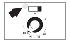
The oven indicator light will glow until the oven has reached the temperature you selected. It will then cycle on and off during cooking.
