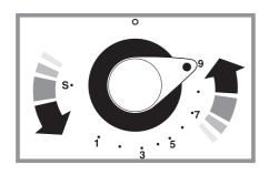
Push in and turn the knob controlling the oven to Gas Mark 9. The oven will light automatically.
