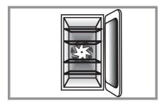
The fan in the oven circulates hot air continuously, which means faster more even cooking.
