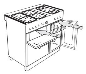
Open the grill door and right hand oven door so that you can get a good grip on the bottom of the fascia panel as you move the oven. Lift the front of the cooker slightly and pull forward.
