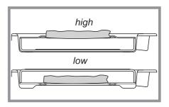
The grill pan grid can be turned over to give two grilling positions.
