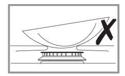
Avoid using unstable and misshapen pans that may tilt easily and pans with a very small base diameter e.g. milk pans, single egg poachers. The minimum pan diameter recommended is 120mm (about 4<sup>3</sup>/<sub>4</sub>").
