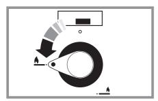
The drawing by each knob indicates which burner that knob controls. Push in and turn a knob to the large flame symbol (\*) and press the igniter button or light with a match.
