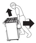
Move the oven a bit at a time, checking behind it to make sure the gas hose is not caught. Make sure both electricity and gas cables have sufficient slack to move the cooker forward as you go along.
