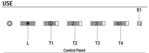
The hood can be switched on pushing directly onto the requested speed without firstly having to select 0/1 button.
