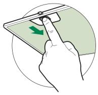
**ATTENTION:** Remove the filters one by one pushing them towards the back side of the hood and simultaneously pulling downwards and towards the centre of the hood (only in case of 60 cm hood version).
