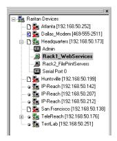
To establish a remote KVM console connection, simply double-click on the KVM path that you would like to control.
