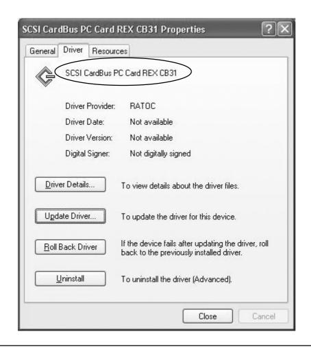
**16.** If you find a **SCSI PC Card REX CB31** under the **SCSI and RAID controllers** on the Device Manager, the CB31U is recognized.
