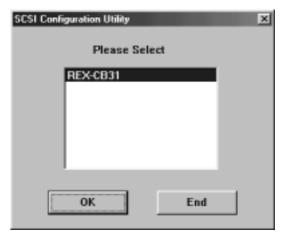
6. SCSI Configuration windows will appear. If you connect FUJITSU MO(M2512A, M2513A), select 10MB/sec.at Translation. If you connect the asynchronous device, select Async. Then click OK.
