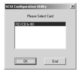
6. SCSI Configuration windows will appear. If you connect FUJITSU MO(M2512A, M2513A), select 10MB/sec.at Translation. If you connect the asynchronous device, select Async. Then click OK.
