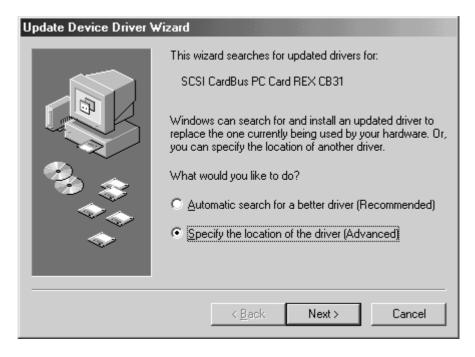
b. When the following window appears, select Search for a better driver than the one your device is using now.(Recommended) and check Specify a location. Insert the floppy disk made in the step 2.
