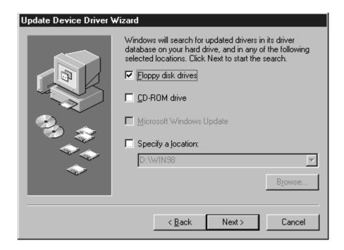
d. When the following window appears, check The updated driver (Recommended) SCSI CardBus PC Card REX CB31 and click Next. If AdvanSys PCI SCSI appears, check One of the other drivers.
