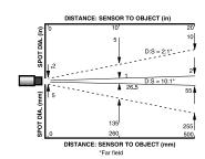
D:S is the optical resolution expressed as a ratio of the distance to the resolution spot divided by the diameter of the spot. Optical resolution for the MID is 2:1 and 10:1. Nominal spot size based on 90% energy.
