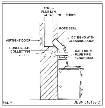
IN ALL TYPE OF CHIMNEYS THE MINIMUM HEIGHT FOR CORRECT OPERATION OF THE CHIMNEY IS 4.5m AND SHOULD TERMINATE ABOVE THE ROOF IN ACCORDANCE WITH REGIONAL STATUTORY REQUIREMENTS RECOMMENDED FLUE DRAUGHT - 12 pa MINIMUM. THE APPLIANCE SHOULD BE INSTALLED AND CONFORM TO THE CURRENT CODES OF PRACTICE FOR INSTALLATION OF DOMESTIC HEATING AND COOKING APPLIANCES BURNING SOLID FUEL - BS 8303.
