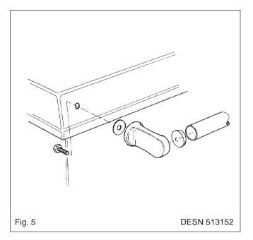
Fit the flue chamber which should be given a 1mm smear of fire cement on the underside then screwed to the cooker. Make sure there is a good seal between the flue chamber and the cooker top (if there is an ingress of air it can affect the flue draught and proper working of the cooker). Before the fire cement hardens remove any surplus with a damp cloth then polish with a dry cloth.
