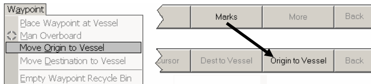
Figure 4-14. Moving the Waypoint You Are Leaving To The Vessel
