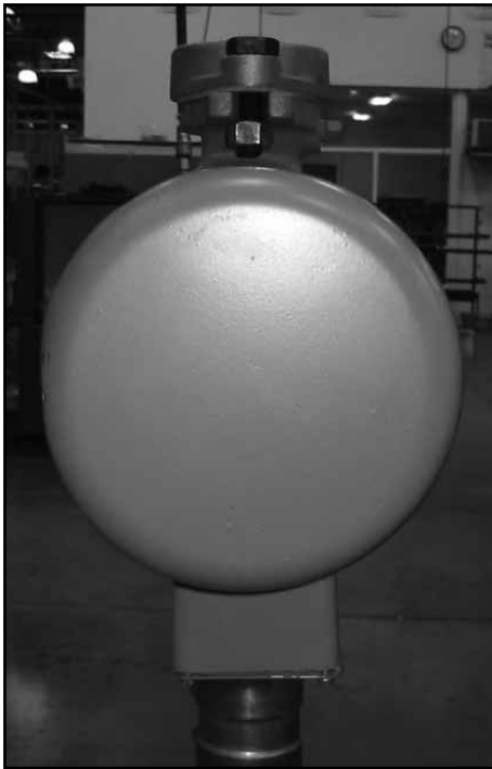
Fig 15: Reposition the pump body so that the electrical box points downward
