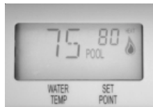
Heating in the POOL Mode
