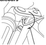
**2** Using a 6mm hex key wrench, tighten both the left and right side handlebar clamps by turning the screws clockwise. When properly tightened, the handlebars cannot be twisted out of alignment.
