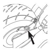
To hook up the brake housing anchor, align the cable guide adjuster and install the spacer and bolt. Do not tighten until final step.
