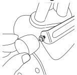
**1** Remove two rubber protectors from fairing mount. Remove two button head screws with rubber washers from both sides of fairing mount.
