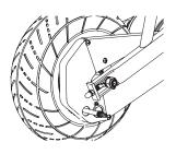
2 Push open the access cover and align the access hole in the drive sprocket with the tire valve. Thread the adapter completely onto the valve and attache the pump and inflate to the PSI indicated on the tire sidewall. Push the access hole cover back.
