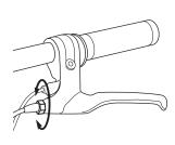
1 To adjust the play, thread the brake lever adjuster in or out 1/4 to 1/2 turn until the desired brake adjustment is attained. Most adjustments are complete at this step. If brake still needs further adjustment, proceed to step 2.
