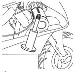
**1** Remove valve extender/adapter from right handgrip.
