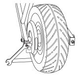
Loosen and remove both axle adjuster nuts.
