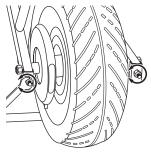
Start screwing on both nuts alternating 1/8 to 1/4 turn at a time until chain is properly tensioned.
