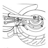
Tighten the brake housing anchor securely. Re-attach the chain guard. Test ride and check. Readjust as needed.
