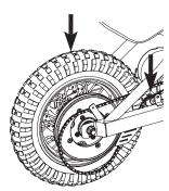
**3** Push the chain tensioner down to loosen the chain and remove the chain from the wheel sprocket and motor sprocket. Push and remove the wheel downward.
