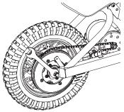
**2** Using two 19mm wrenches, loosen both axle nuts.
