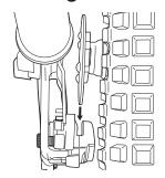
1 Position wheel in front fork and slide disk brake into caliper.
