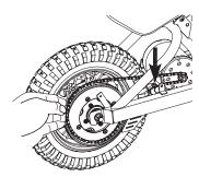
4 Install the new chain or wheel by slipping the chain around the axle. Slide the axle into the slots on the frame. Slide the chain tensioner down and maneuver the chain onto the rear sprocket and front sprocket.
