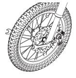
**3** With a 14mm and 17mm open wrench tighten the front wheel screws.
