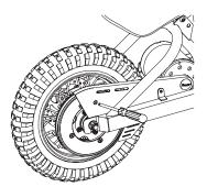
**1** Loosen screw and remove chain guard.
