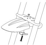
**1** Align fender with the hole in the fork and insert the bolt. Tighten securely using a 10mm open wrench and 5mm Allen wrench.
