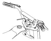
**2** Align parallel to the fork and tighten the bolts using a 6mm Allen wrench. When properly tightened, the handlebars should not move forward or back.
