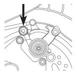
**3** If the brake rotor is dragging on the brake pads, use your fingers to twist the caliper adjuster in either direction until rotor is centered between pads.
