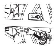
**2** If brake is too tight or has too much slack, use a 10mm wrench to loosen the nut for additional adjustment on the brake cable on the rear wheel. Securely tighten nut when done.
