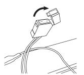
**2** Locate fuse box on top of battery. Open the fuse cover to expose the fuse.
