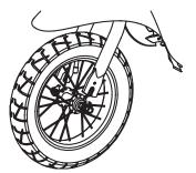
**2** Insert the wheel into the front fork with the lock washers on the outside of the fork
