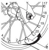
**2** Start with spoke closest to tire valve and tighten each nipple. In sequence, exactly 1/4 to 1/2 turn. A single 1/4 to 1/2 turn may not be enough to bring the spokes into proper tension. Continue tightening all spokes no more than 1/2 turn in sequence until all spokes are tight
