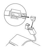
**3** Remove the fuse and replace with a new one of equal amperage.
