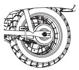
**7** Tighten the brake housing anchor securely.
