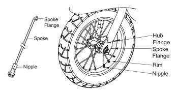
1 Verify spoke tension by grasping and shaking each spoke. Spoke should not be loose from hub. Look for any play between spoke flanges where it mates with hub. Try to turn nipple using your fingers. You should not be able to spin any nipple by hand. If one or more spokes are loose, or if you can turn any nipple using your fingers, all spokes must be checked and need to be tightened with a spoke wrench.
