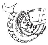
**4** With two 15mm wrenches, loosen the axle. Slide the wheel forward to loosen the chain and remove the wheel. Note the sequence of the hardware.
