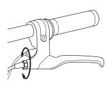
**1** To adjust the play, thread the brake lever adjuster on the hand brake in or out 1/4 to 1/2 turn until the desired brake adjustment is attained. Most adjustments are complete at this step. If brake still needs further adjustment, proceed to step 2.
