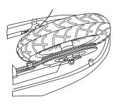
**5** Install the new chain or wheel by slipping the chain around the axle. Slide the axle into the slots on the frame. Slide the wheel forward and maneuver the chain onto the rear sprocket, motor shaft and chain tensioner.
