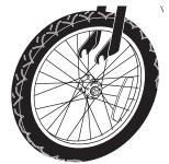
2 Remove wheel and replace tire. To reinstall wheel, reverse these steps.
