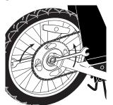
2 Loosen rear axle by attaching wrenches to both axle nuts and loosening counter-clockwise. Pull chain off sprocket and remove wheel from frame.
