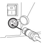
1 Plug the charger port into the port on the scooter. The charger works with the power switch in either the on or off position.
