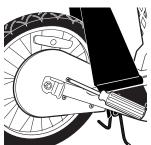
1 Remove chain guard with Phillips Screwdriver.
