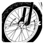
1 Loosen front axle by attaching 10/15 mm wrenches to both axle nuts and loosening counter-clockwise.
