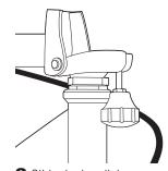
**3** Slide the handlebar stem down into the front fork until it fits snuggly into the lock nut on the headset.
