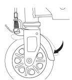
**2** Squeeze the hand lever to test the brake to make sure it is working properly. The front fender should clamp down and rub against the front wheel. If brake is not working properly, proceed to the next step.
