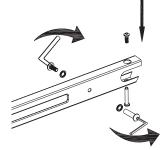
**1** Remove black plastic protector at the end of the frame. Using two 5mm hexagonal wrenches, remove the two hexagonal bolts and the two coupling bolts from the frame.
