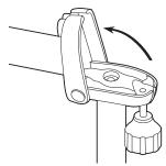
**1** Remove the plastic protector covering the wedge and loosen the black folding knob and swing to the 6 o'clock position to unfold the handlebar stem.
