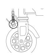
**3** If the brake is too tight or too loose, use a 8mm open wrench and a 3mm allen wrench to make adjustments as needed.
