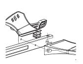
**2** Remove black plastic protector at the end of the platform. Position the right and left foot platforms up to the frame and align holes.
