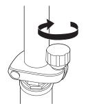
**6** Swing the black folding knob to the 12 o'clock position and tighten by hand until handlebars are secure.
