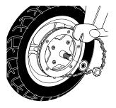
**5** Pull the wheel out. Note the arrangement of the hardware sequence.
