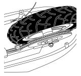
**6** Install the new chain or wheel by slipping the chain around the axle. Slide the axle into the slots on the frame. Slide the wheel forward and maneuver the chain onto the rear sprocket, front sprocket and chain tensioner. Tighten the axle nuts.
