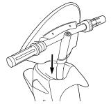
**2** Insert handlebar assembly into the fork until it stops. Raise to desired height, keeping the stem and fairing aligned within the red arrows of the safety zone.
