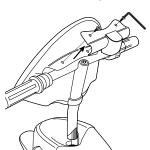
**1** Loosen the two hexagonal bolts with the 3mm hexagonal wrench and remove the plastic handlebar cover.
