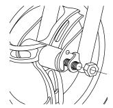
**3** Insert the tab on the lock washer into the hole on the front fork and tighten the nuts with the supplied wrench.
