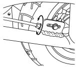
**2** If the brake lever adjuster is threaded outward and the brake still has too much slack, use the rear brake adjuster for additional adjustment.
