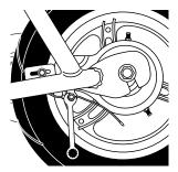
**8** Re-connect the brake cable and tighten the brake cable anchor.
