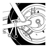
**7** Tighten the brake housing anchor securely.
