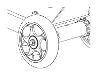
**3** Make sure the locknut, spring washer and small washer are securely tightened against the wheel.
