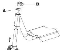
**1** Remove the black protective cover from the top of the fork. Using a 13 mm wrench, loosen collar clamp bolt and slide collar clamp (B) up the fork and remove. Remove washer (A) from fork. Insert the front fork into the steering tube. Slide washer (A) back onto the front fork. Slide collar clamp (B) back down onto the fork until it is sitting directly on top of washer (A).
