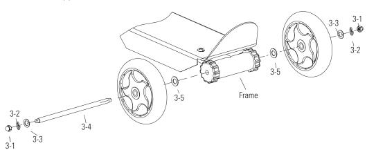
**1** Remove the locknut, spring washer and washers (x3) **from one side** of the axle bolt. Insert the axle bolt through the rear wheel. Insert the large washer (3-5) onto the axle bolt between the frame and rear wheel and slide the axle bolt through the frame. Slide the other large washer and wheel onto the axle bolt. **Note:** Wheels are interchangeable.
