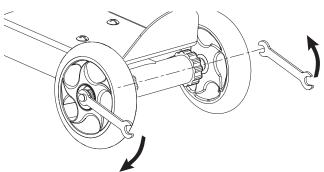
**2** Insert the small washer (3-3), spring washer (3-2) and locknut (3-1) onto the axle bolt and tighten securely using two (2) 10 mm wrenches.
