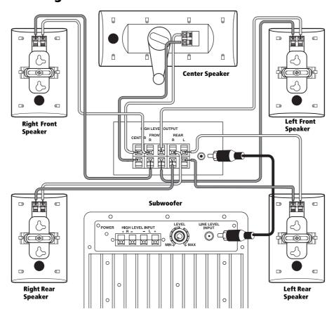
Your amplifier/receiver's line out jacks might be labeled either REC OUT or PRE OUT. In that case, connect the subwoofer's **LINE LEVEL INPUT** jack to the amplifier/receiver's line out jack with phono (RCA) cables (not supplied). If your amplifier/receiver has "STEREO OUT" for subwoofer, connect with dual-to-single (RCA) cable (not supplied).
