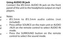
Suggest using Ø3.5mm AUDIO IN jack for MP3 player and AUX IN jacks for auxiliary equipment such as DVD, VCR or PC. If the AUX IN (or AUDIO IN) audio signal is mono, you may not receive audio on all speakers.
