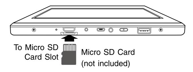
Insert the micro SD card into the tablet's Micro SD slot until it clicks.
