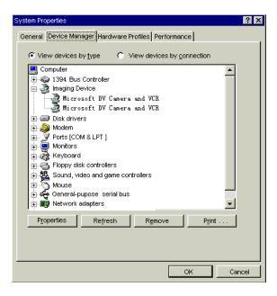
Note: The AVT-2050 and the camcorder can be detected only when they are powered on. If powered down, system will delete them automatically.
